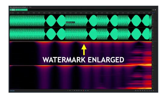
While I applied the watermark only to the beginning of the test file, it can be applied to the entire file, to any section of the file, or at a repeating interval. The process is straightforward and offers great flexibility in how it is used to implement a solid authentication method.
